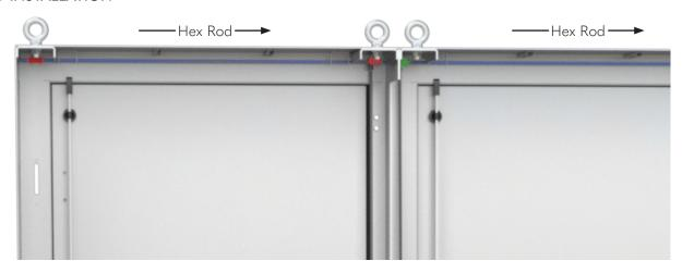
Step 3: Slide the hex rod (shown in blue) horizontally into the next enclosure. Captured within Figure D, the hex rod will then protrude approximately halfway into the other hex rod adapter (shown in green) of the adjacent enclosure. The new hex rod will now link up to the corresponding rod just installed.
