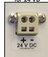
Electrical connection for 24 VD
